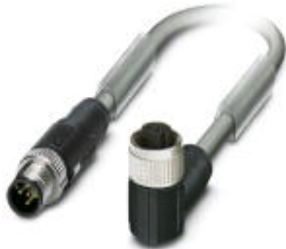
Bus system cable, CANopen®, 5-position, PUR halogen-free, Gray RAL 7001, shielded, Plug straight M12-SPEEDCON, A-coded, on Socket angled M12-SPEEDCON, A-coded, Cable length: 15 m
